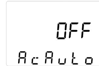
1. The above figure shows AC function setting interface of tower UPS (tower UPS can be set through the panel).
