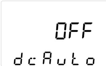
1. The above figure shows DC function setting interface of tower UPS (tower UPS can be set through the panel).
