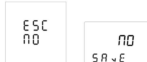
1. The left figure shows “save setting” interface of rack UPS, and the right figure shows the inverter no-load shutdown function setting interface of tower UPS.
