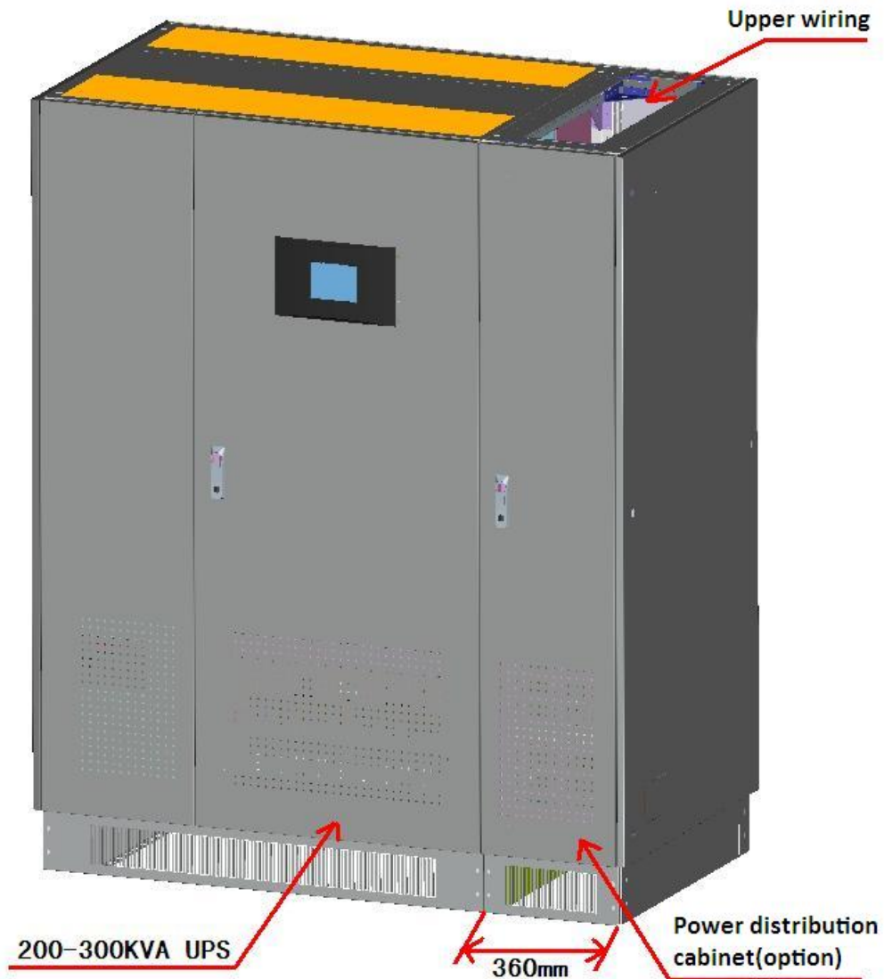
Figure 38: Diagram for installation of UPS and power distribution cabinet
