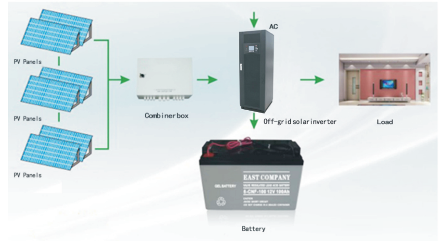
Fig 1 Composition of Off-grid Photovoltaic System
