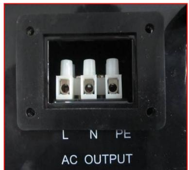
Step 2: Insert stripped AC cables of appropriate size into the cable glands. Fix the phase cables into corresponding terminals with screwdriver according to marks. Fix ground cable into the ground terminal.
