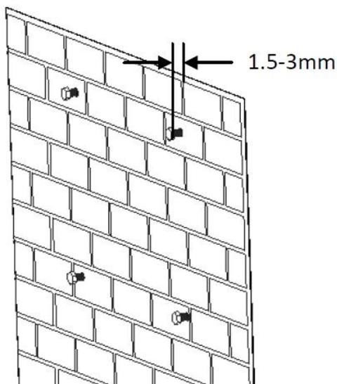
c) Attach the inverter to the screws downwards slightly.
