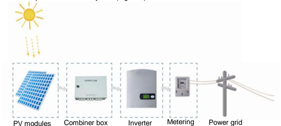
Figure 1 PV grid-connected system
